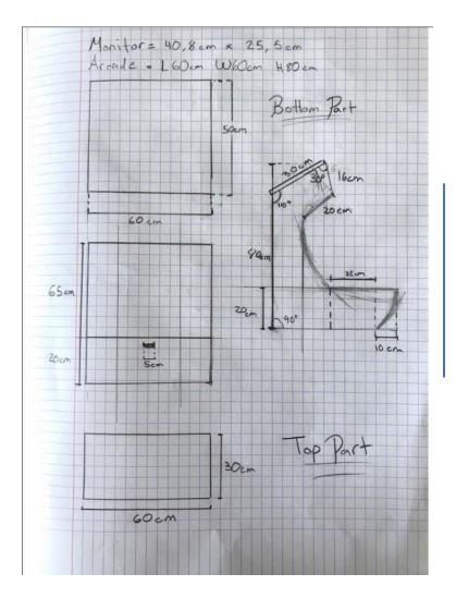
We went for an immersive design. As you can see from the sides, it has a ship shape with the logo of the game in the front. The arms of the arcade are 10 cm longer than the control center (machine's joystick and buttons), to give a feeling of being inside a ship
